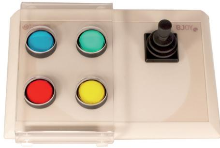
This mouse is based on a joystick similar to the wheelchairs' one and big accessible buttons. It is part of the BJOY range of products, which means its hardware can be tailored to each user's needs and capabilities and its operation customized using the BJOY Configurator Software. BJOY Stick-A has been especially designed for people with little strength in their arms.
